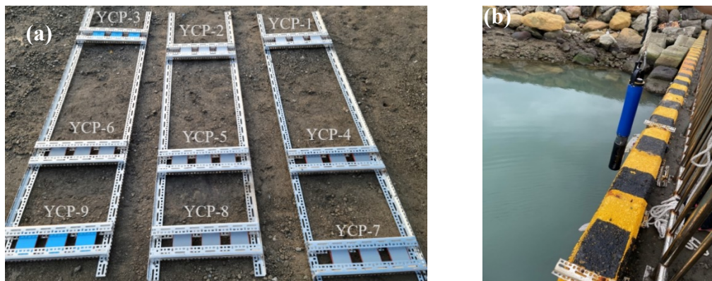
圖 1 (a) 海水吊掛實驗初始試片分佈圖，(b) 多參數水質儀。 Figure 1 The initial distribution of specimens in the seawater hanging experiment, (b) water quality testing instrument.
