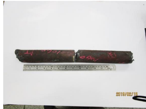
圖 6 斷裂之冷風管樣品外觀。 Figure 6 The appearance of the fracture cold air tube sample.
