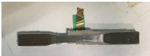
圖 4 均勻腐蝕試片表面圖 Figure 4 Specimen used for accelerated general corrosion.
