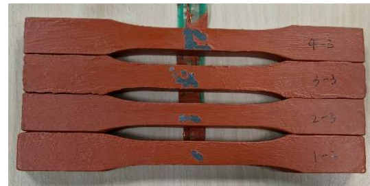
圖 6 局部腐蝕試片表面圖 Figure 6 Specimens used for accelerated localized corrosion.
