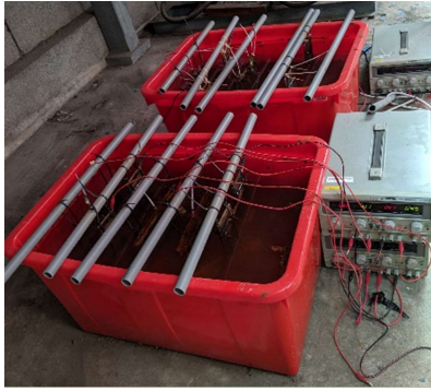
圖 7 加速腐蝕實驗架設圖。 Figure 7 Accelerated corrosion test setup.
