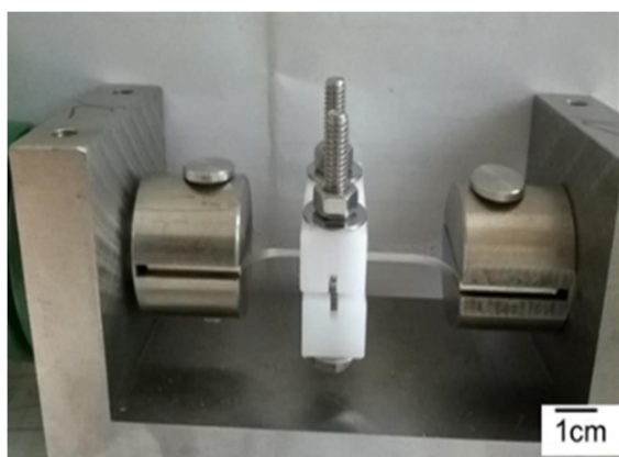
圖 2 應力腐蝕治具與試片尺寸。 Figure 2 The dimensions of SS 304L tensile test specimen and crevice former under tensile stress.
