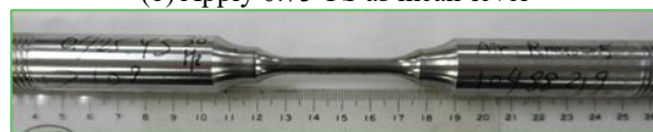
(c) 施加應力中值為 0.725 降伏應力 (c) Apply 0.725 YS as mean level
