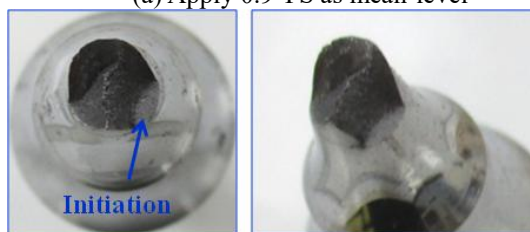
(b) 施加應力中值為 0.75 降伏應力 (b) Apply 0.75 YS as mean-level
