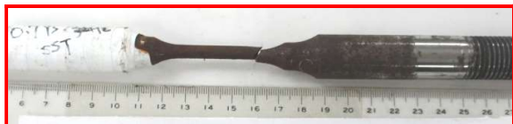
圖 4 施加應力中值為 0.7 YS 於 30Hz 荷重頻率之腐蝕疲勞試驗後外觀。 Figure 4 Corrosion fatigue at 0.7 YS mean-level stress and 30 Hz loading frequency.
