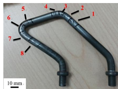
圖 2 引擎蓋掛耳 NG 件金相取樣位置。 Figure 2 Metallographic sampling position of NG hood hook.
