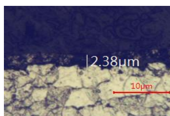
圖 9 CNT/SPHC 金相剖面圖(放大倍率:500 倍)。 Figure 9 Metallographic cross-sectional observation of CNT/SPHC (Magnification:500 times).
