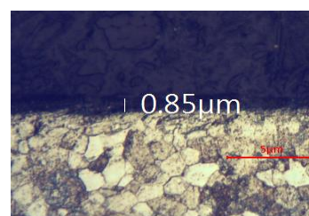
圖 10 Cr/SPHC 金相剖面圖(放大倍率:500 倍)。 Figure 10 Metallographic cross-sectional observation of Cr/SPHC (Magnification:500 times).
