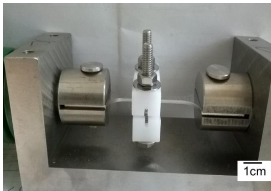
圖 1 間隙腐蝕試片與間隙形成裝置之耦接墊片。 Figure 1 The dimensions of: (1) SS 304L specimen and (2) crevice former device.
