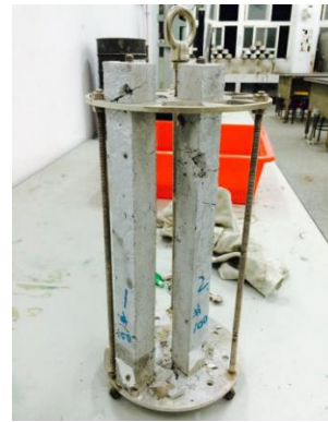
圖 5 滾筒渣 100% 取代量砂漿棒斷裂示意圖。 Figure 5 Schematic diagram showing cement mortar stick rupture by replaced 100% baosteel slag short flow.
