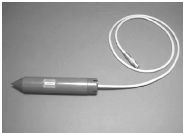
圖 10 AC 腐蝕偵測電極。 Figure 10 Appearance of AC corrosion probe for underground pipelines.
