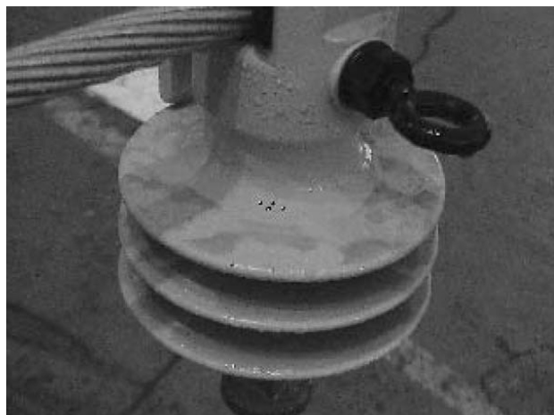
圖18 放電影像觀測污損液附著情形。 Figure 18 Artificial contaminants figure in UV corona image monitoring.
