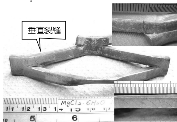
圖 16. 304SS 網板經應力腐蝕模擬試驗 16 小時後的外觀 Fig.16 Appearances of 304SS expanded metal specimens after stress corrosion cracking simulation test for 16hrs.
