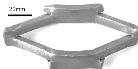
圖 18. 固溶化處理的 304SS 網板，經應力腐蝕模擬試驗 30 天後的外觀 Fig.18 Appearance of a solution treated 304SS expanded metal specimen after stress corrosion cracking simulation test for 30 days.
