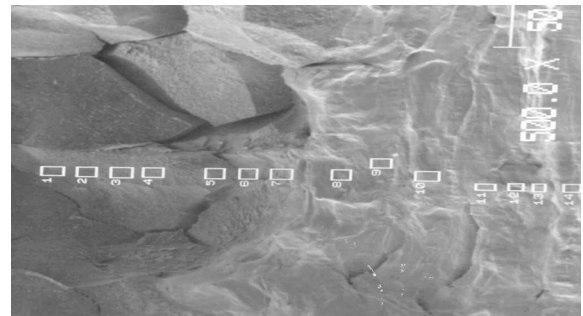
圖7. A31-b 裂縫上分析鉻元素濃度分佈 Fig. 7. The analysis of Cr concentration on A31-b crack front by AES.
