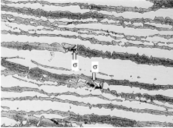
Figure 10 Precipitation of sigma, ( phase observed in the low temperature heat affected zone. (× 400 Magnification)
