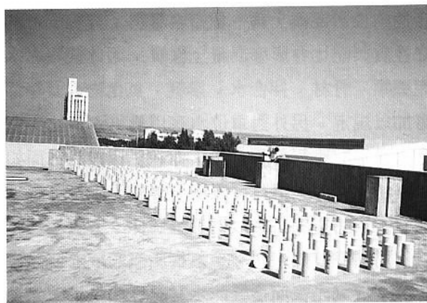
圖一 港灣技術研究大氣曝露試體擺置情形 Fig.1 The natural weathering exposure station, Institute of Harbor and Marine Technology, R.O.C. (2)
